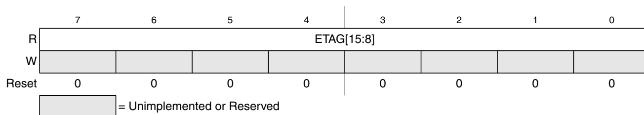
Figure 26-18. EEE Tag Counter High Register (ETAGHI)
