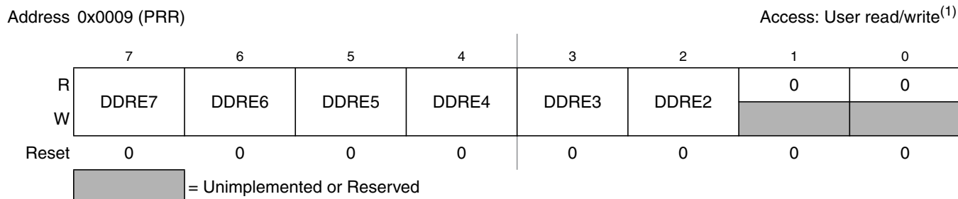
Figure 2-10. Port E Data Direction Register (DDRE)
